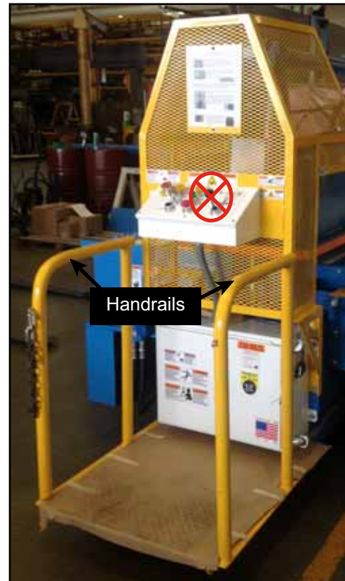
Figure 6-8: Hold Handrails for Support, NOT Joystick
