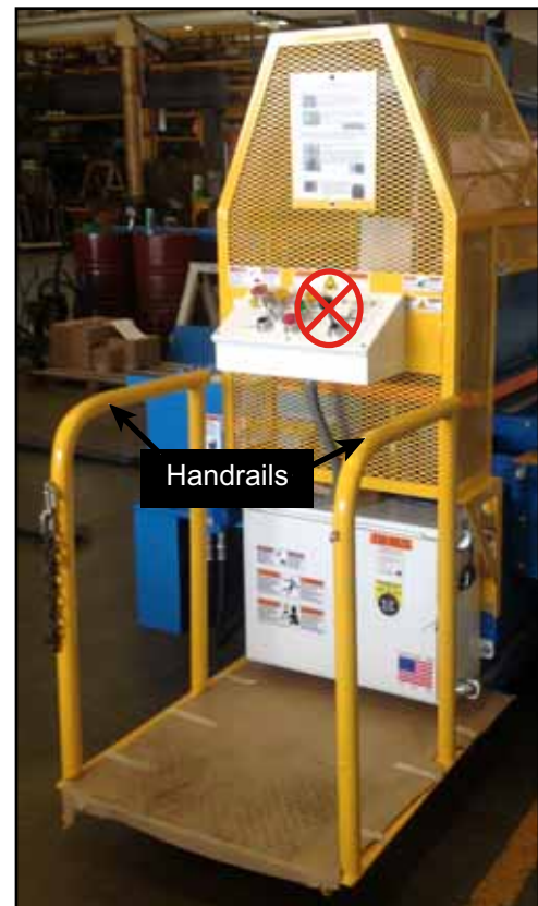
Figure 6-5: Hold Handrails for Support, NOT Joystick
